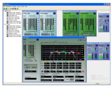
network of devices. One more click and you can monitor all the devices in the network using MonIcons. Click one of these and you can control the device. Plug another device into the network and see it being automatically added to PodWare.
