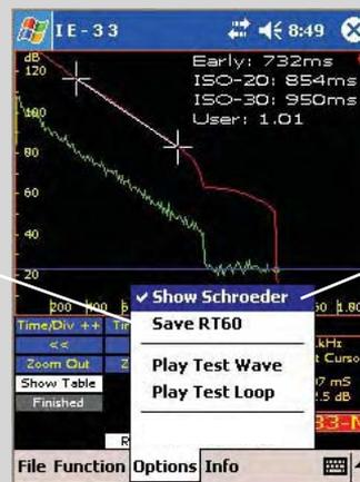
Displays the Schroeder curve (in red). This applies a smoothing algorithm to the Decay curve. If desired, the Cursors may be placed on this curve instead of the actual decay curve.
