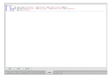
To use the trigger page, left-click on the 'create' button at the bottom-left of the screen. After naming the new trigger, 'Allways Do Nothing' will appear in red text to the right of the name of the trigger, and the minus and insert icons. The minus icon will collapse the trigger definition into a single line with a name, and a plus icon will replace the minus. To expand the definition, left-click on the plus icon, and the full definition will display.
