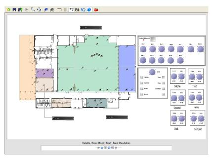
In addition to reflecting the state of the system, the run/simulate feature also allows the user to manipulate elements of the system to test logic changes. Switches can be pressed, selectors actuated, doors opened and closed, and levels changed. With each user change, the system will evaluate logic changes and reflect those changes to the layout graphically.
