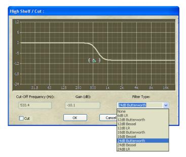
gain, and filter type. Frequency and gain can be entered through the keyboard, and filter type through a pull down menu. These values can also be input by dragging the shelf point with the mouse, and using the wing tool. Use the cut checkbox in the lower-left corner of the dialoge to select cut v.s. shelf filtering. As with other dialogs, the user can bypass the processing block with the bypass check box.
