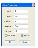
Options in this dialog are: ratio, floor, threshold, release off gain, NOM enable, and last on.
