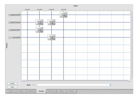
When a mode has been selected, and the y-axis populated with outputs, the grid is ready for a full cross-point routing matrix for that mode. To place a routing point, left-click on any cross-point, and the point will appear. To remove the point, left-click the point again, and it will disappear.
