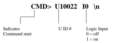
U ID numbers are assigned at the time a control is created in the Sonata software. These U ID numbers are unique to each control in a Sonata layout file, and can be found in the properties dialog box for a given control. These ID numbers are automatically assigned during control creation in the software, but can be manually changed when desired. The U ID numbers are used to match physical controls in the real world with virtual controls created in software.
