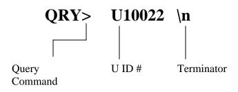
iFlex controls always contain a switch, an output, and a level control. This means that for each unique U Id# there will be an associated switch, and output, and a level. This does not mean that users will always use the three elements for a given U Id #, and often users will only create one of the elements of a control per U Id #. The iFlex mixer will, however, always return the states of all three elements for a given U Id # request.
