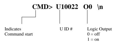
U ID numbers are assigned at the time a control is created in the Sonata software. These U ID numbers are unique to each control in a Sonata layout file, and can be found in the properties dialog box for a given control. These ID numbers are automatically assigned during control creation in the software, but can be manually changed when desired. The U ID numbers are used to match physical controls in the real world with virtual controls created in software.
