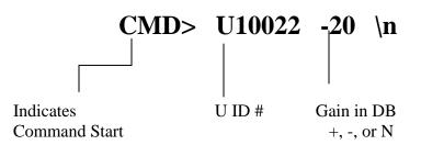
U ID numbers are assigned at the time a control is created in the Sonata software. These U ID numbers are unique to each control in a Sonata layout file, and can be found in the properties dialog box for a given control. These ID numbers are automatically assigned during control creation in the software, but can be manually changed when desired. The U ID numbers are used to match physical controls in the real world with virtual controls created in software.
